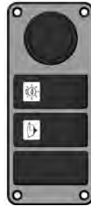
Figure 2. 480 BR and 480 Sport control panel
